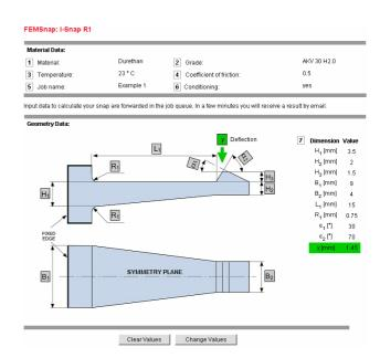
Figure 3 Form after start of calculation
