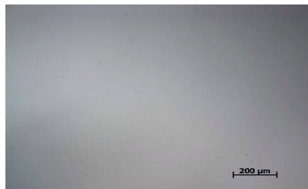
Fig. 1 Film surface without anti-block agent
