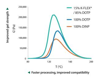
Using a blend of 15% of a K-FLEX<sup>®</sup> dibenzoate plasticizer with 85% of DOTP (a common non-phthalate GP plasticizer), gel strength and processing times were significantly improved in contrast to DOTP or DINP alone.
