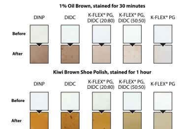
Fused vinyl tiles prepared with K-FLEX<sup>®</sup> dibenzoate plasticizers exhibit superior stain and extraction resistance compared to films made using common phthalates and non-phthalate alternatives.
