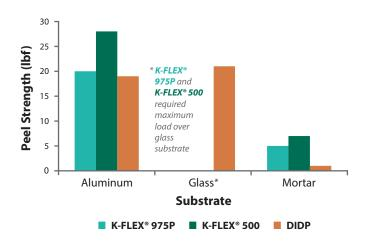
K-FLEX® 975P and K-FLEX® 500 demonstrated excellent adhesion-in-peel performance in a silyl terminated polyether sealant formulation in contrast to DIDP, a commercial phthalate.
