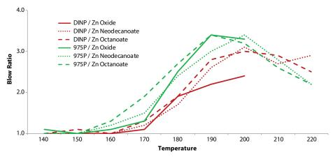
Figure 1. Effect of various kickers in chemically blown foam utilizing either DINP or K-FLEX® 975P plasticizers. Substitution of DINP with K-FLEX 975P can result in a 42% reduction in foam density while reducing processing [or foam blow] temperatures by 5%.
