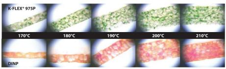
Figure 2. Cross section of foam blow utilizing K-FLEX® (top) and DINP (bottom) plasticizers. K-FLEX plasticizers allow the vinyl leathercloth to achieve a low density, fine, uniform cell structure at lower temperatures.
