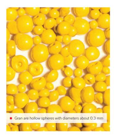
A new era in coloring plastics has begun with Macrolex®, one of the first microgranulated dyes ever. It is
