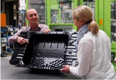
The load compartment well can withstand high mechanical stresses and is around 30% lighter than comparable sheet metal designs.
