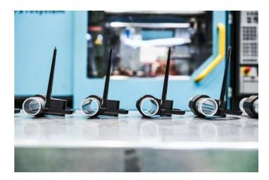
Demonstrator components produced at LANXESS using the hollowprofile hybrid technology. They are characterized by a high degree of torsional stiffness and strength.
