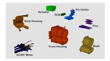
The concept provides for a modular design of the charging inlet. Once the cables and contact pins have been placed in the holder and the PCB has been clipped in, all the charging inlet components are put together with the aid of snap fits.
