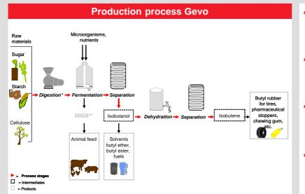
\* Mechanic, chemical und enzymatic; \*\* DDGS – Distillers' Dried Grains with Solubles 8
