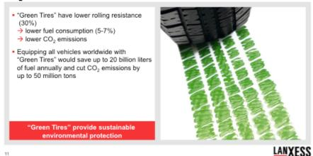
Their biggest advantage is that they reduce rolling resistance – without cutting corners on safety. And less rolling resistance means lower fuel consumption and lower emissions.
